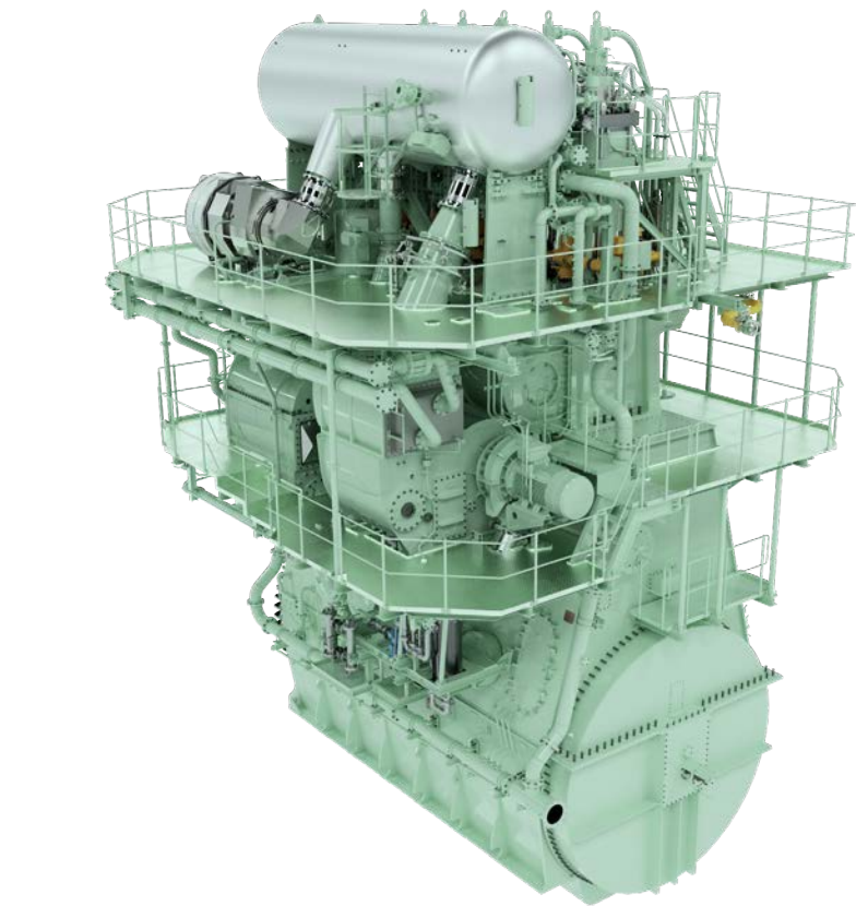
Fig. 5: EGR installation on ME-GA engine
