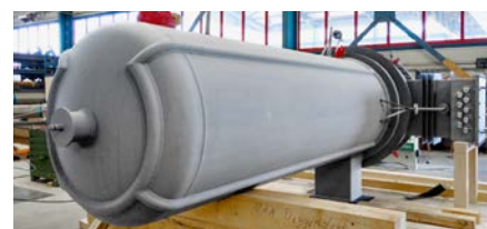
Fig. 4: MAN Energy Solutions electric salt heaters used in MOSAS long-duration energy storage
