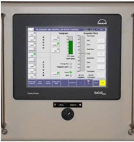
Fig. 22: LOP-P with telegraph receiver and propeller pitch control
