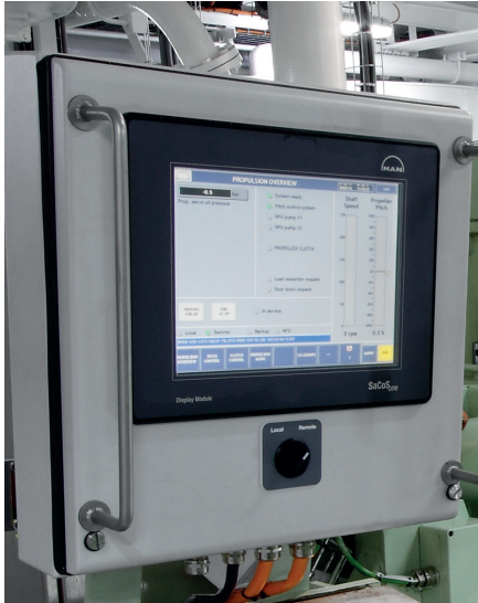
Fig. 54: Cabinet with local operator panel for propeller (LOP-P) – placed on four-stroke engine
