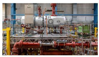
Heat pump unit on the test bed
