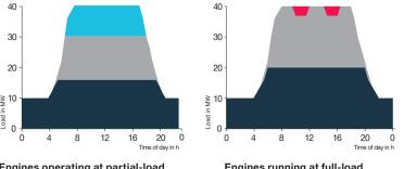
Engines operating at partial-load to meet the reserve requirements.
