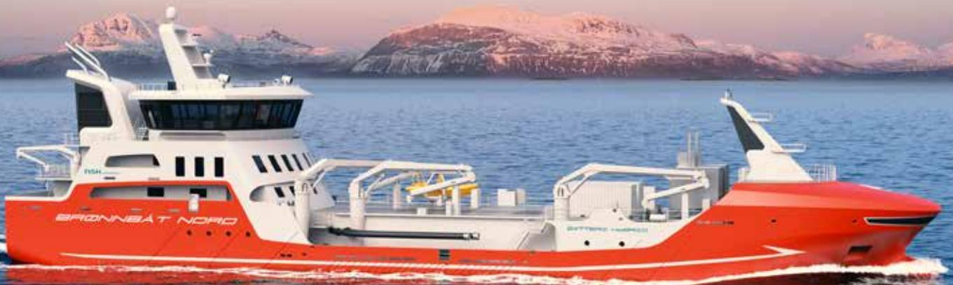
*Rendering of the new 2,800 m<sup>3</sup> – 79.3 x 16m battery hybrid wellboat (image courtesy of NSK Ship Design)*
