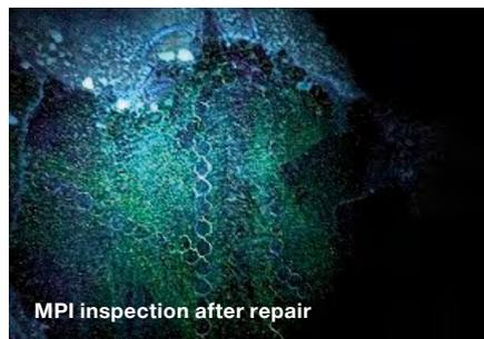
MAN PrimeServ On-site Recovery is certified by Lloyd's Register to perform the Metallock metal stitching procedure. It is a cold process for recovering broken, cracked or otherwise damaged cast iron or aluminium, while eliminating thermal stress and resultant component distortion.
