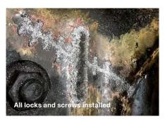
MAN PrimeServ On-site Recovery is certified by Lloyd's Register to perform the Metalock metal stitching procedure. It is a cold process for recovering broken, cracked or otherwise damaged cast iron or aluminium, while eliminating thermal stress and resultant component distortion.
