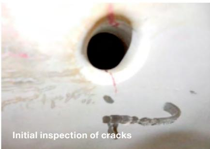
Initial inspection of cracks
