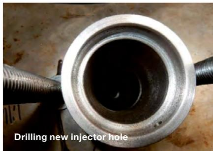
Drilling new injector hole
