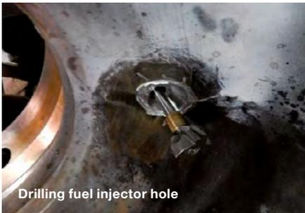
Drilling fuel injector hole
