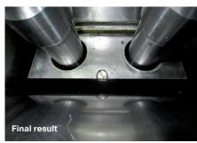
When heat from a bearing failure has altered the geometry of the main bearing saddle, a complete dismantling of the engine, line-boring and reassembly is usually needed, taking the engine out of service for as much as six months.
