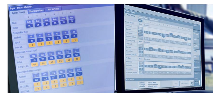
PMI Offline will Show an automatic calculation of Effective Power, Mean Indicated Pressure Pi, Compression Pressure Pcomp, Maximum Pressure Pmax and Scavenge air pressure Pscav. It also gives a graphical presentation of PT, PV and balance diagrams, together with Pmean and Pmax, and calculates proposals for fuel pump index adjustments.
