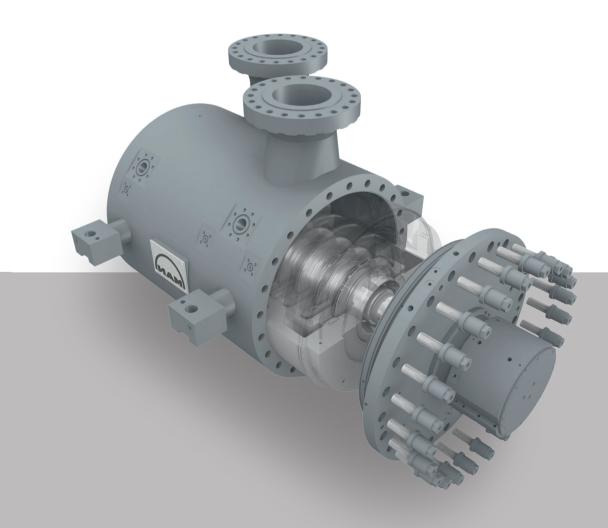
The MAN Energy Solutions barrel type compressor is a single-shaft centrifugal compressor for applications in Oil & Gas, HPI/CPI, petrochemical processes and gas transport. Its cost effective design comes in various frame sizes. Inlet flow rates range from 200 to 230,000 Am<sup>3</sup>/h and discharge pressures go up to 800 bar.
