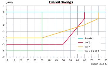
Fig. 2: Fuel oil savings [g/kWh]
