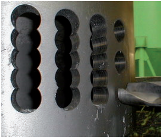
Figure 7: Drilling of scavenge air ports.
