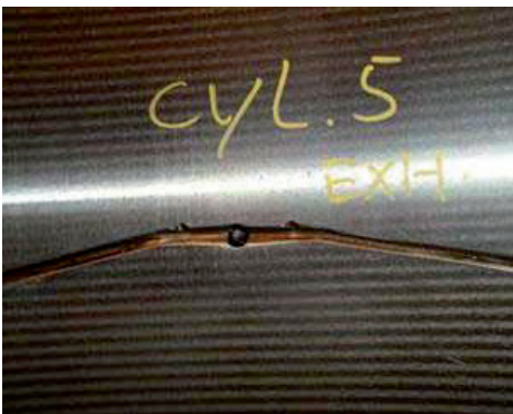
Figure 14: Lubricator deep straight groove (in combination with a zig-zag groove).
