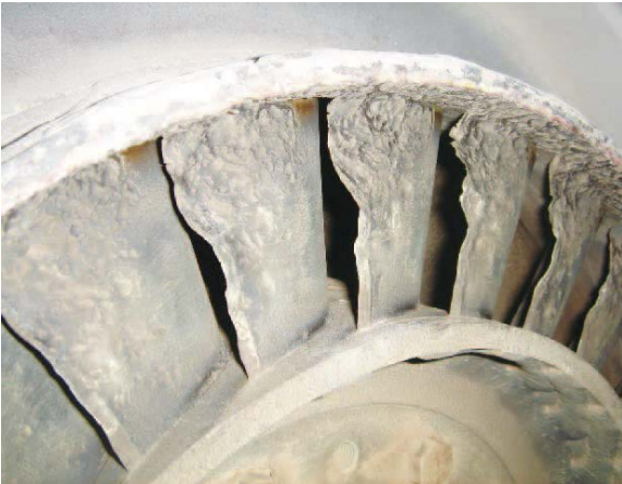
Damaged nozzle vanes
