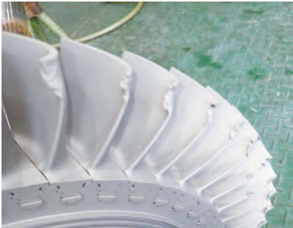
Damaged turbine blades
