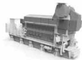
PTO on front end – external pump
