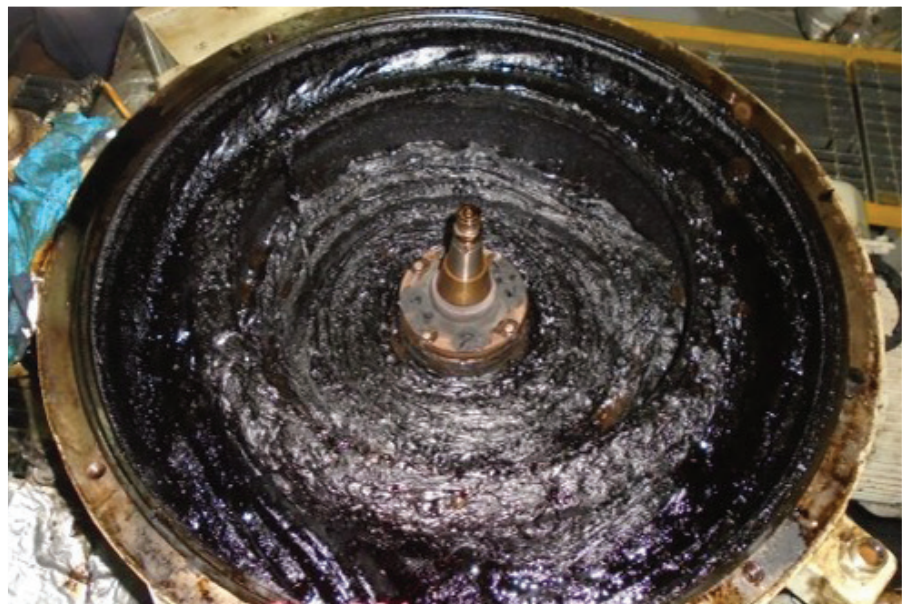
Fig. 34: Heavy sludging and block separators as a result of either unstable fuel or incompatibility between two fuels.
