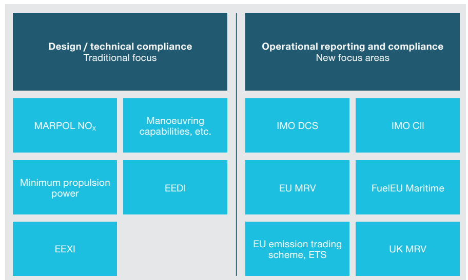
Fig. 7: Design and operational compliance scheme grouped
