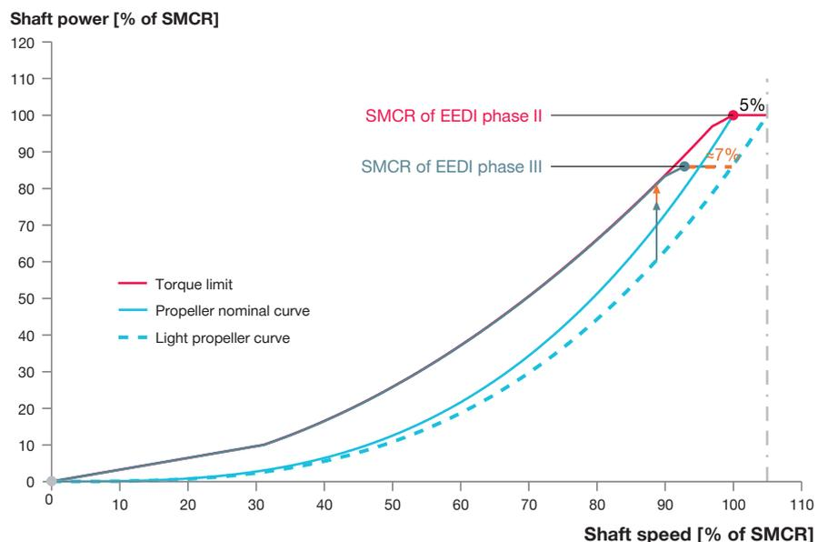
Fig. 13: Increased LRM by SMCR speed reduction
