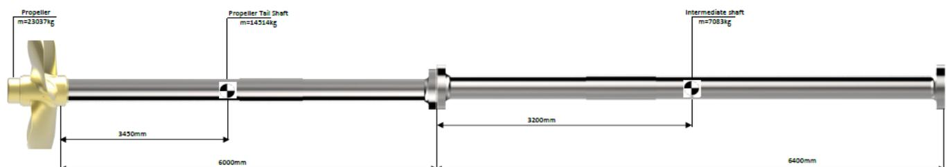
Fig. 9: Shaft line of the propulsion plants
