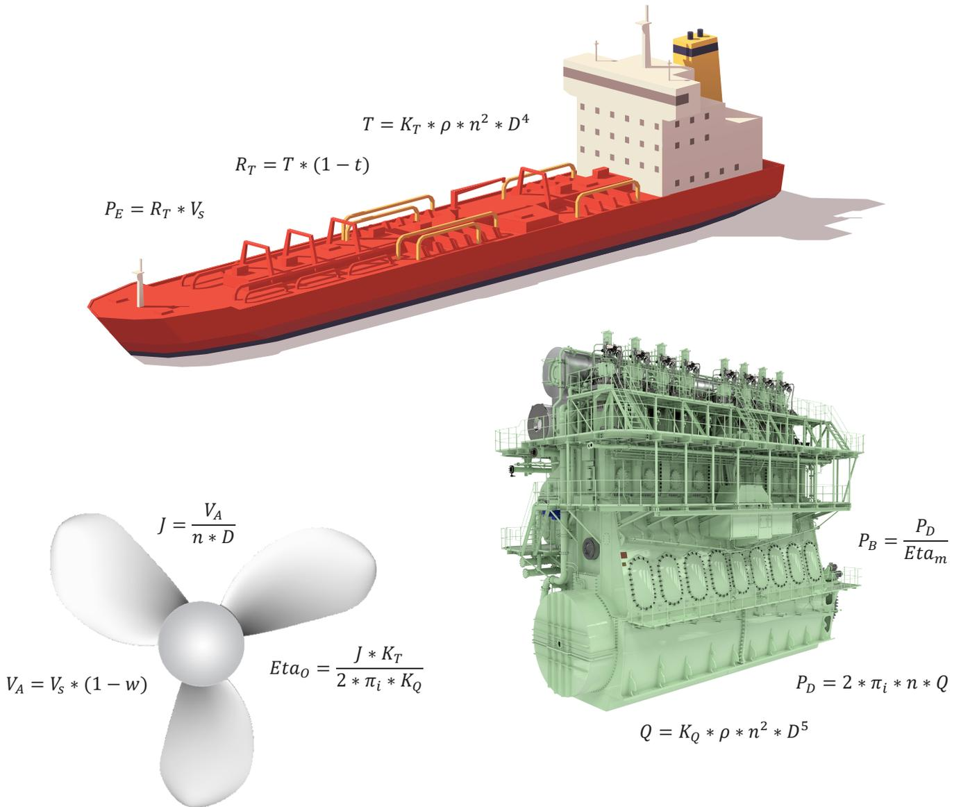
Fig. 2: Hull-engine-propeller matching (source: [www.friendship-systems.com](http://www.friendship-systems.com))
