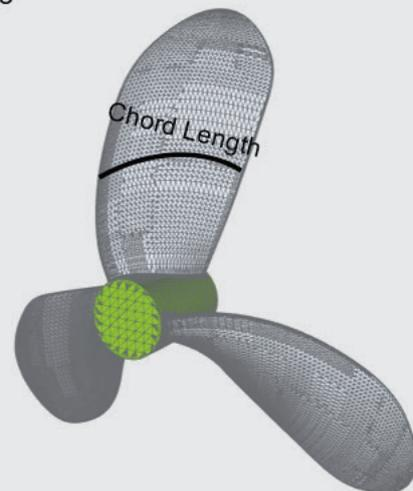
Fig. 10: Blade chord length for the propellers with four and three blades (source: [www.friendship-systems.com](http://www.friendship-systems.com)) [5]
