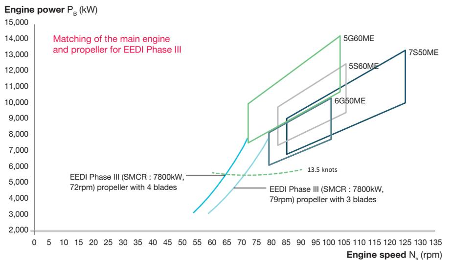
Fig. 5: EEDI Phase III with optimum propeller speeds
