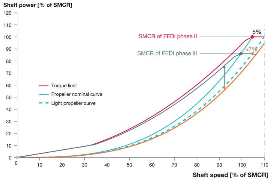
Fig. 14: Increased LRM by propeller pitch reduction
