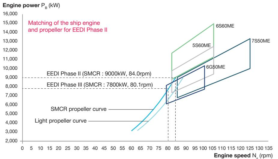
Fig. 4: EEDI Phase II propeller curves and engines available
