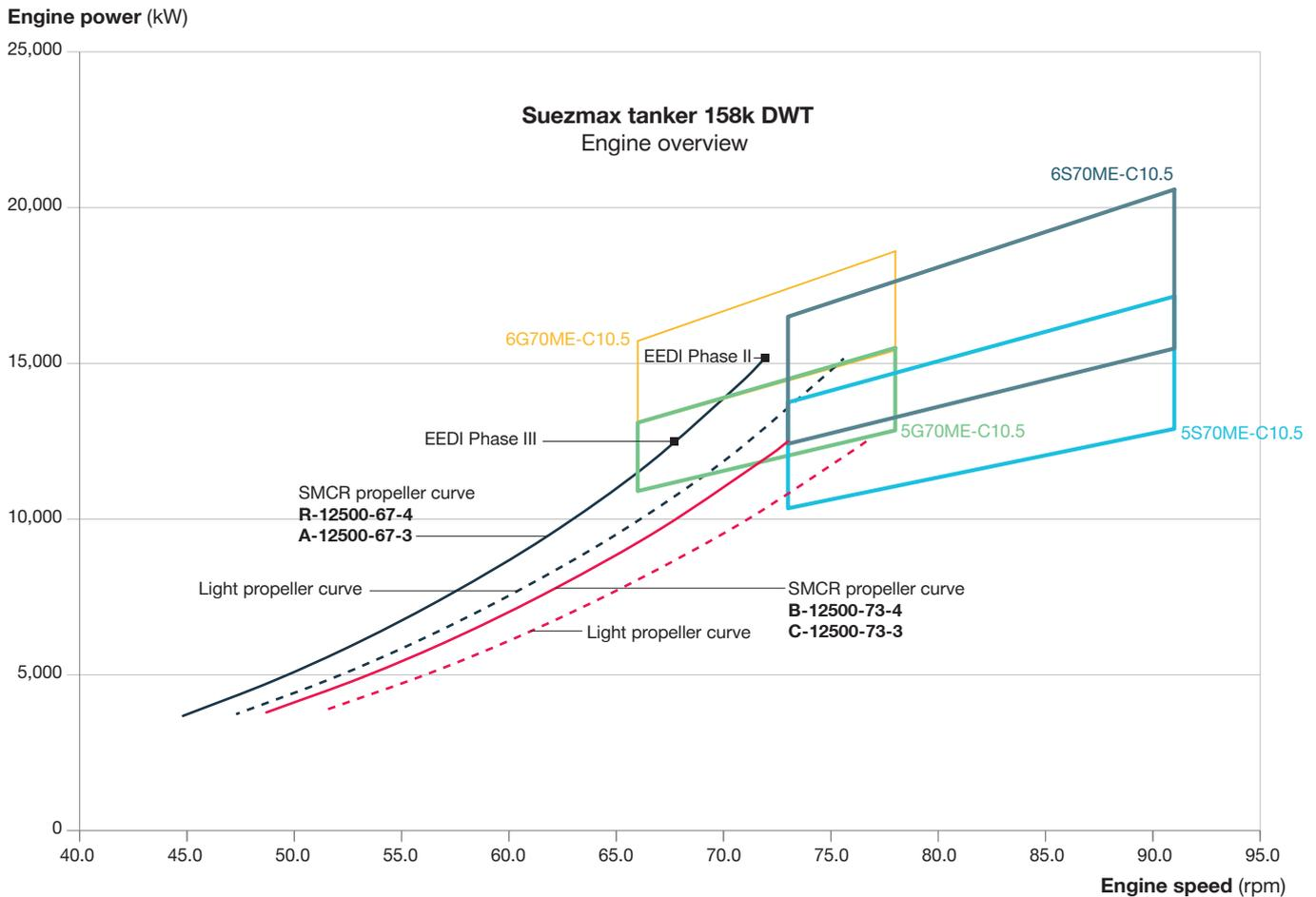
Fig. 11: Matching of available engine and propeller variant for EEDI Phase III
