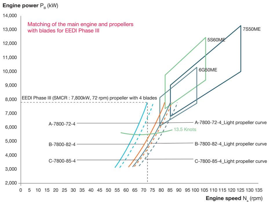
Fig. 7 Variants with four propeller blades
