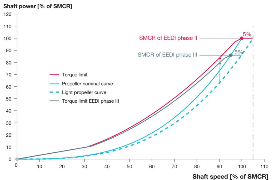
Fig. 12: Absolute margin between the light propeller curve and the torque limit
