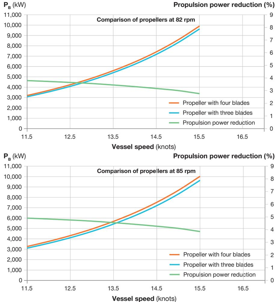
Fig. 8 : Propulsion power difference in the ship speed range
