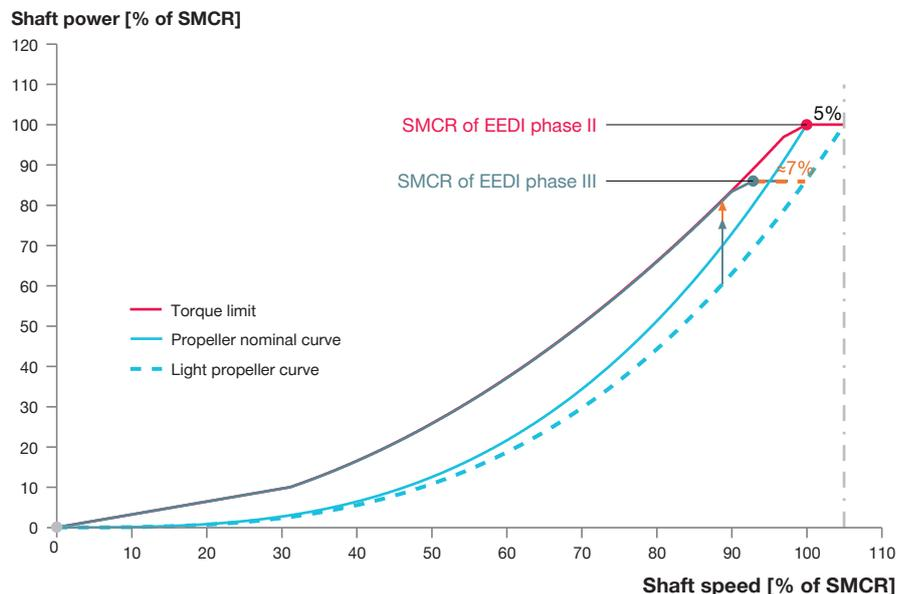
Fig. 13: Increased LRM by SMCR speed reduction
