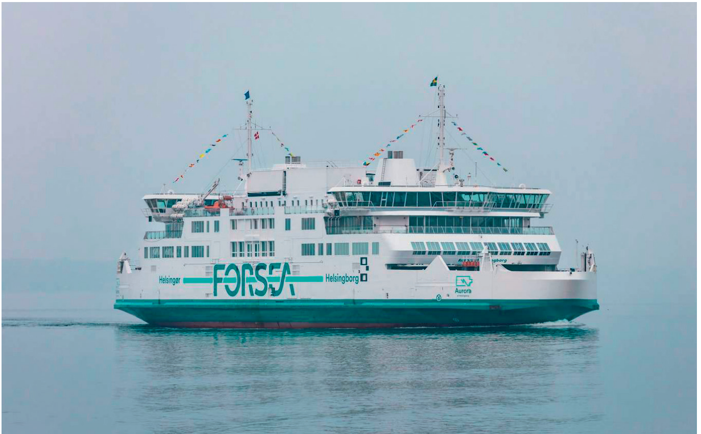
Fig. 1: Aurora , one out of two of the world's largest battery-electric ferries as of 2019, operating on the 2.5 nautical mile route between Elsinore, Denmark, and Helsingborg, Sweden. Courtesy of ForSea
