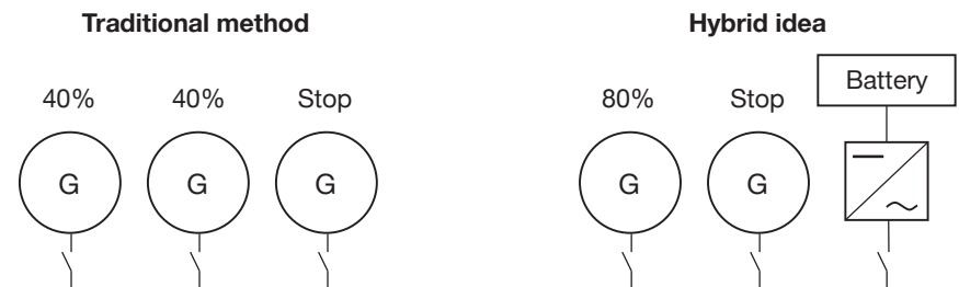
Fig. 18: Illustration of operating principle during critical operations with and without battery
