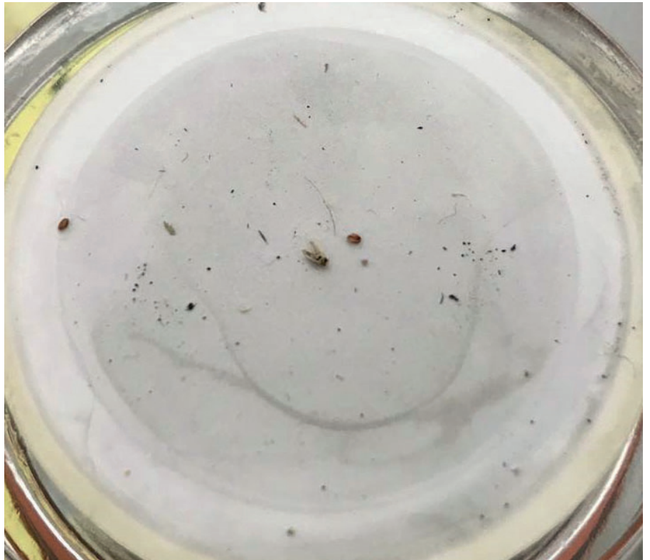
Fig. 23: Example of too dirty filter disc
