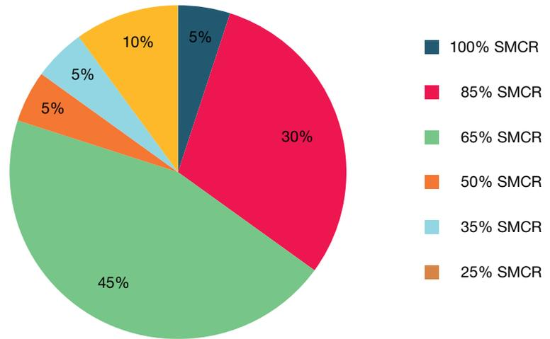
Fig. 7: Load profile for the time at sea
