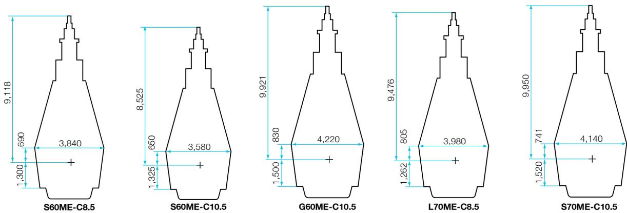
Fig. 1: Main dimensions of possible main engines, all measurements in mm
