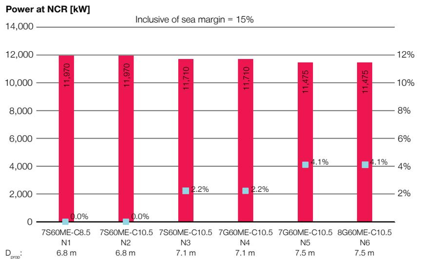
Fig. 10: Expected propulsion power demand at NCR = 85% SMCR for 19 knots
