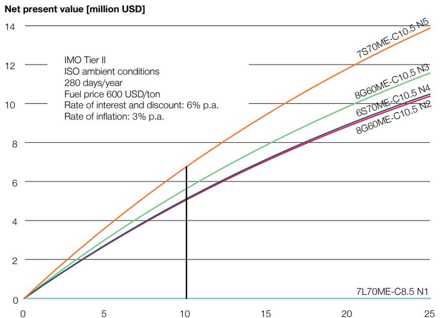
Fig. 9: Saving in main engine operating costs (NPV) for 21 knots without (above) and with EcoEGR (below)
