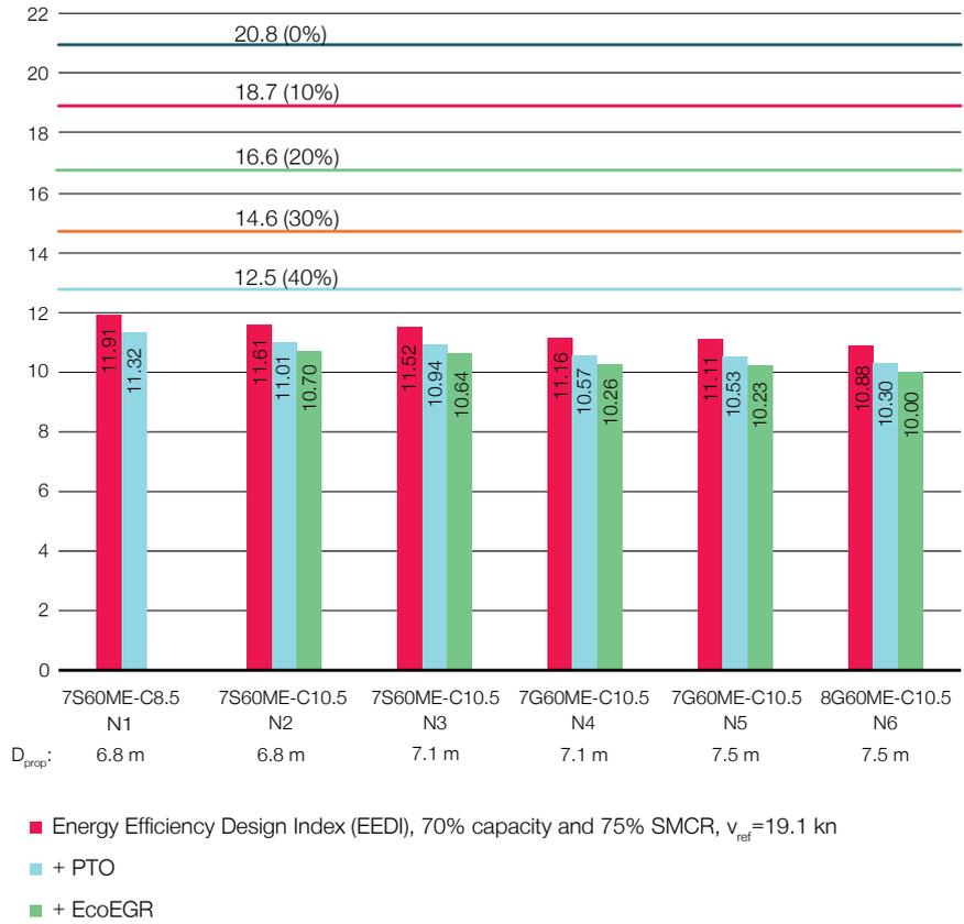
Fig. 13: Required and attained EEDI at 19 knots for MDO
