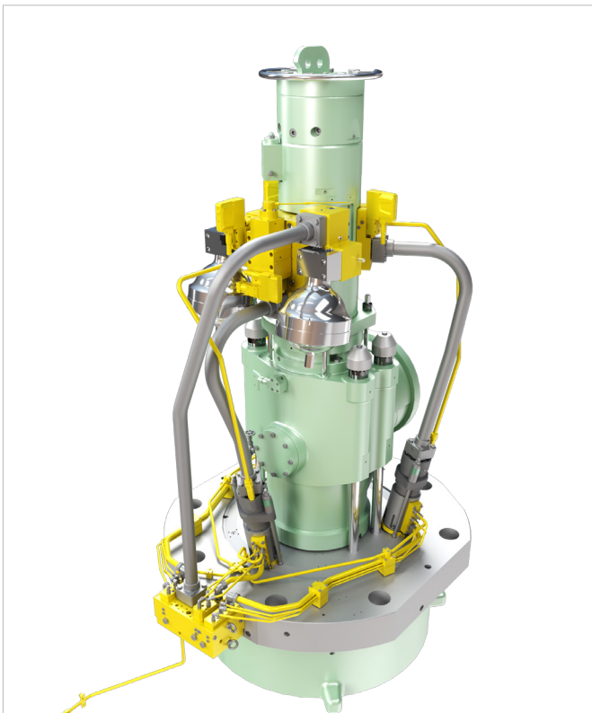
Fig. 30: Sequential injection system with integrated top-controlled exhaust valve
