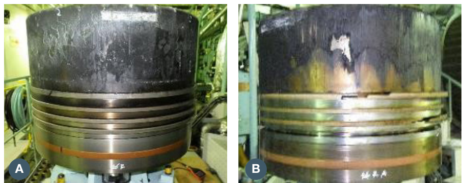
Fig. 15: Comparison between A. a four-ring pack and B. a three-ring pack on an ME-GI engine. The cleanliness is improved by changing the ring pack.
