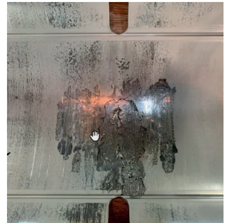
Fig. 41: Crosshead bearing centre suffered fatigue damage on G50ME-C engine
