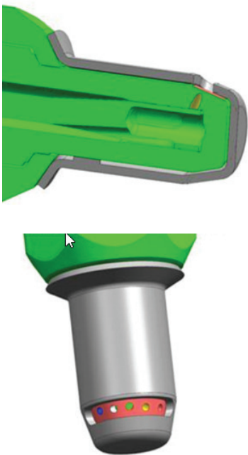
Fig. 9: LGIM gas nozzle with heat shield for G95-LGIM engines
