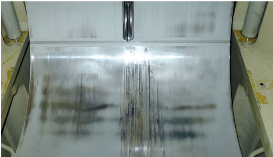
Fig. 41: Crosshead bearing centre suffered fatigue damage on G50ME-C engine
