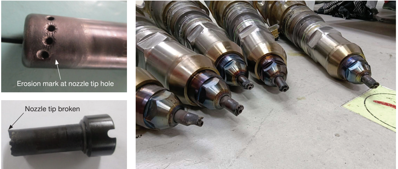
Fig. 8: Nozzle failure after a period of Tier III operation with water addition
