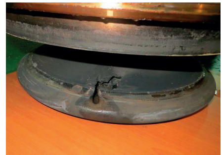
Fig. 36: Blow-by from the seating area
