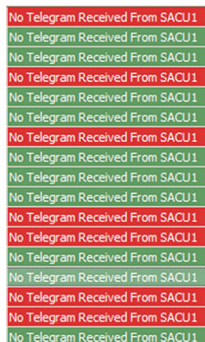
Fig. 51: Missing telegram alarms causing gas shutdown on dual-fuel engines
