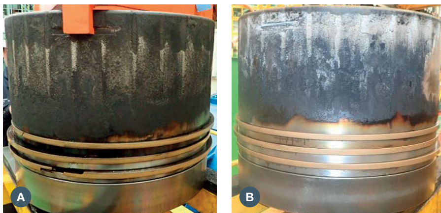
Fig. 14: Condition after test bed when A. using a low-BN cylinder oil, B. using a 70-BN cylinder oil. Notice the difference in the piston ring land cleanliness.
