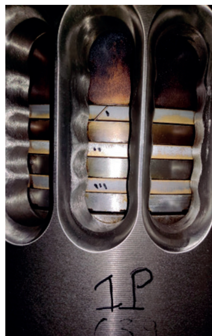
Fig. 25: Cylinder condition after 8,000 running hours – remaining running-in coating is yellow (G70ME-C10.5-GI)
