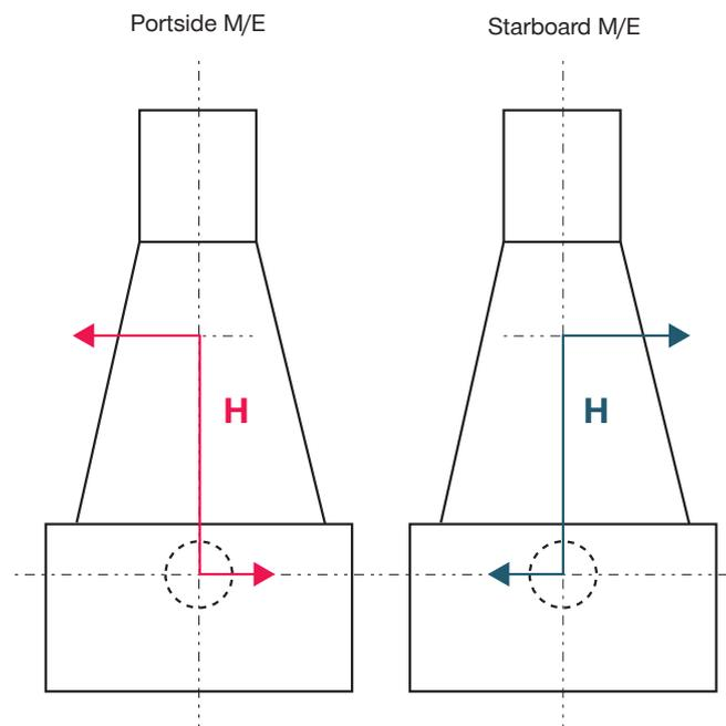
Fig. 3: Synchronised guide force moments (synchro phase = 0 deg.)
