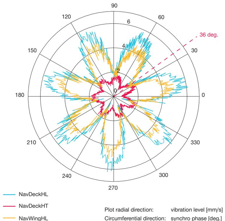
Fig. 9: 5G70ME-GI engine at 64 rpm, optimal phase = 36 deg.
