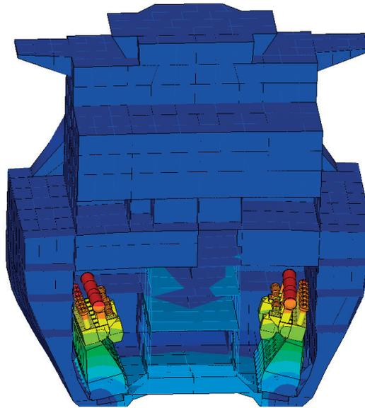
Fig. 2: Engine and hull vibration system on an LNG carrier subjected to main engines guide force moments.
