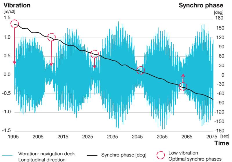
Fig. 6: Navigation deck – longitudinal direction (LNG carrier 2017)
