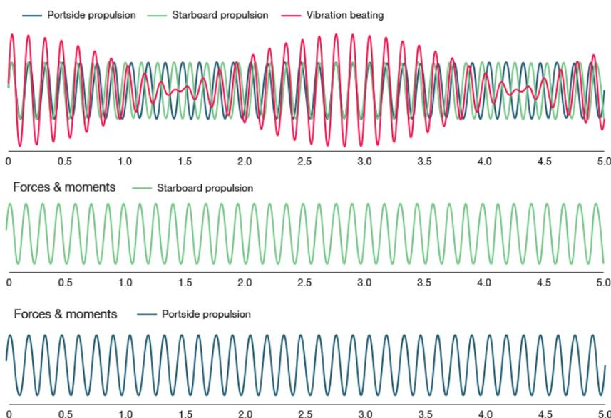
Fig. 4: Vibration beating in a non-synchronized twin propulsion system
