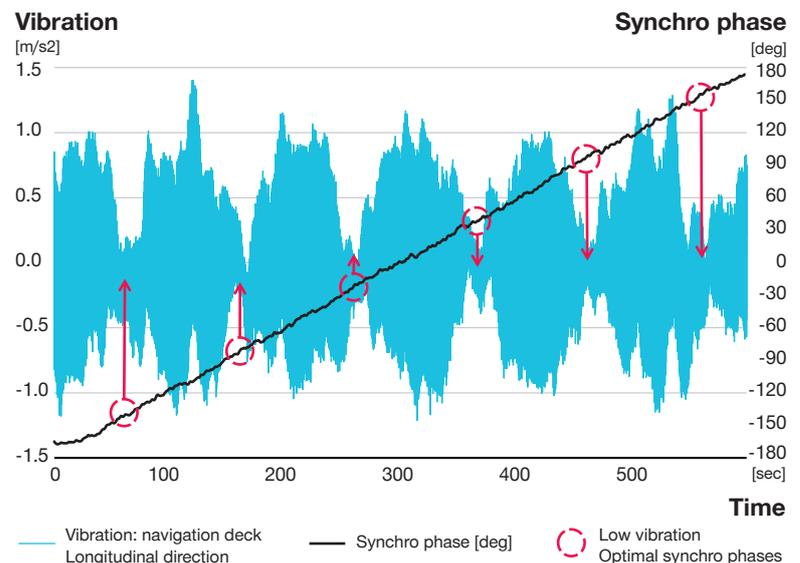
Fig. 7: Navigation deck – longitudinal direction (LNG Qflex 2006)
