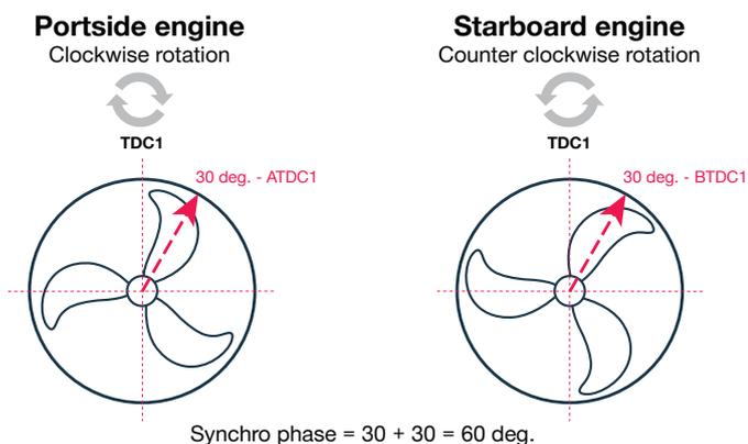
Fig. 5: Definition of synchrophase (example 60 deg.)
