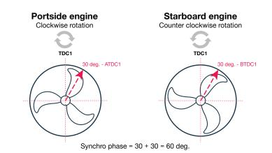
Fig. 5: Definition of synchrophase (example 60 deg.)
