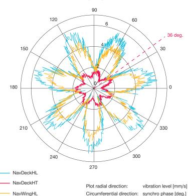
Fig. 9: 5G70ME-GI engine at 64 rpm, optimal phase = 36 deg.
