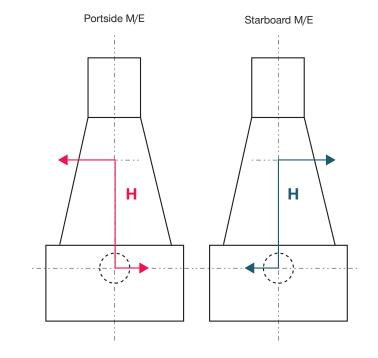
Fig. 3: Synchronised guide force moments (synchro phase = 0 deg.)
