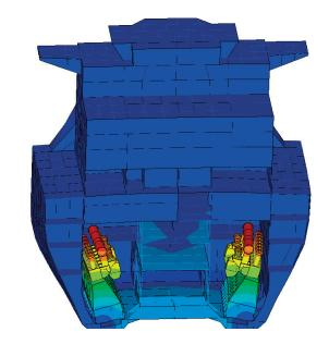
Fig. 2: Engine and hull vibration system on an LNG carrier subjected to main engines guide force moments.
