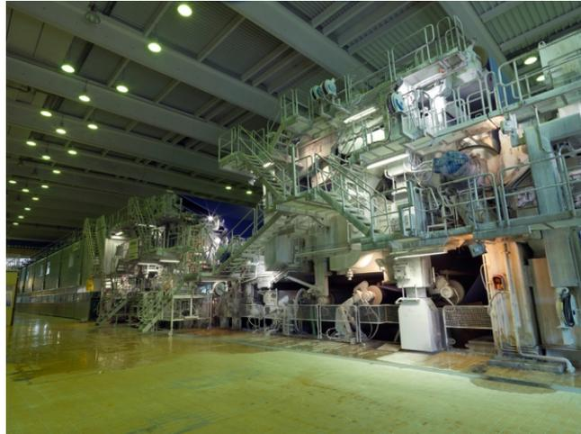
*UPM's PM3 paper machine mainly produces uncoated fine paper weighing 60–120 g/m<sup>2</sup>*
