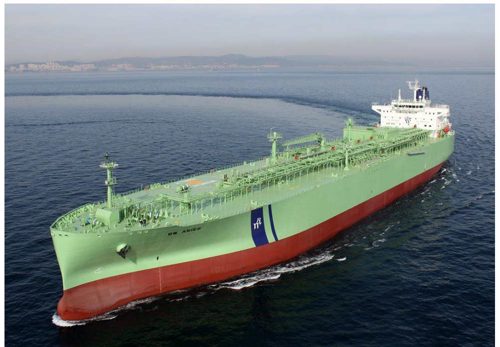
An example of BW LPG's modern fleet, the 'BW Aries' from 2014 is an 84,196 m 3 VLGC (picture courtesy BW LPG)
