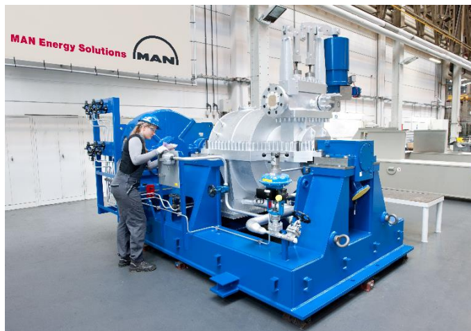
MAN steam turbine during assembly
