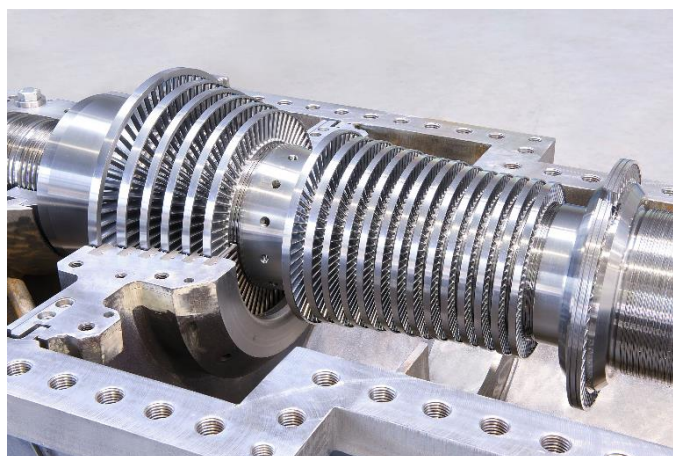
MAN steam turbine rotor
