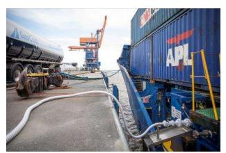
The 'ElbBLUE' has reduced its greenhouse gas (GHG) emissions by 27% by operating on a blend of climate-neutral, synthetic natural gas (SNG) and conventional liquefied natural gas (LNG), compared to LNG alone.
