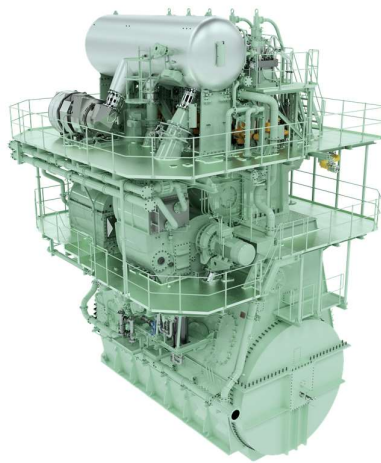
Graphical rendering of an MAN B&W two-stroke engine with EGR system
