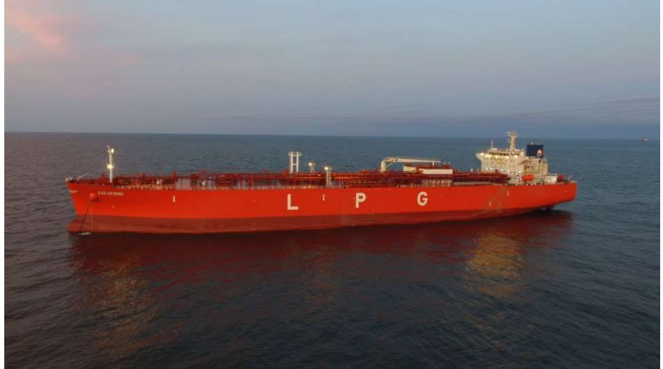
The 'Gas Gemini' will see its MAN B&W 6G60ME-C engine converted to a dual-fuel MAN B&W 6G60ME-LGIP capable of running on LPG
