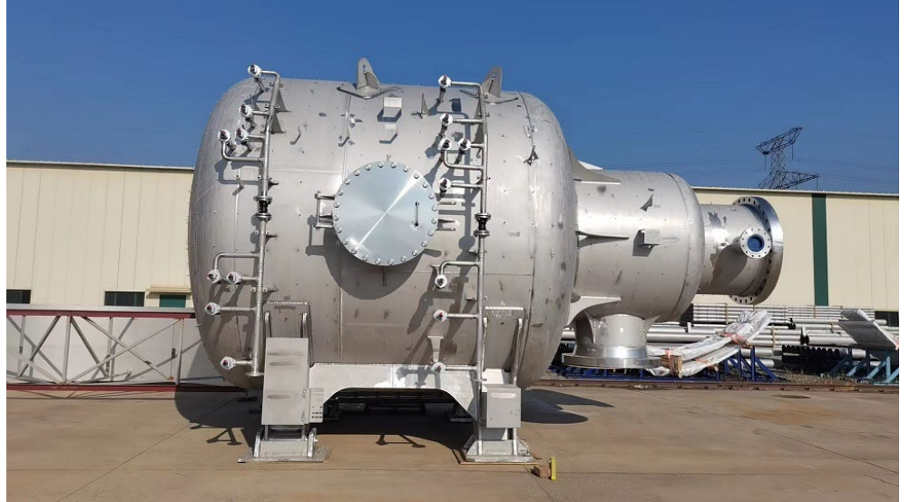
The Cluster 5 Double Layer has a diameter of 3,900 mm and a total weight of 28 metric tons
