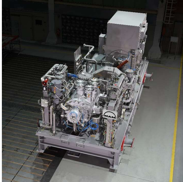
A centrifugal compressor train for offshore gas production by MAN Energy Solutions
