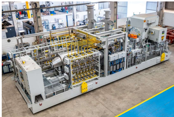
A screw compressor train as offshore Vapour Recovery Unit (VRU) by MAN Energy Solutions
