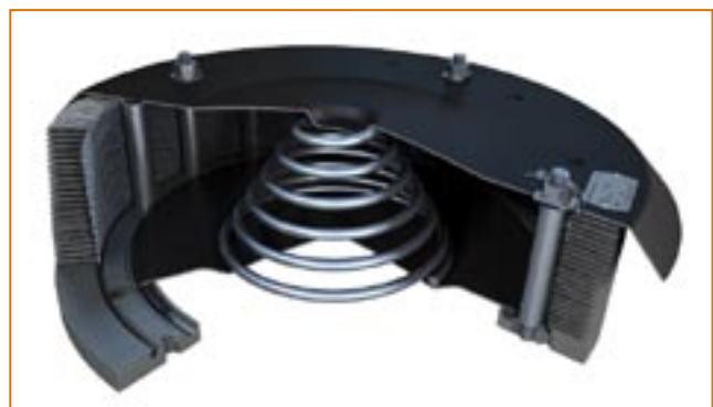
Fig. 1: Example of crankcase explosion relief valves type approved in 1999.
