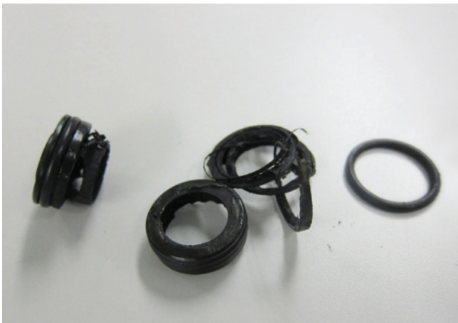
Damaged synthetic piston (POM: Polyacetal)
