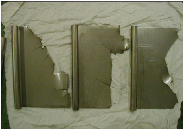
Fig. 2: Broken flap valves
