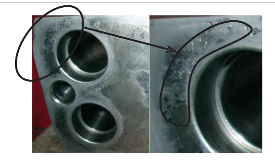
The above picture shows an example of fretting marks at the assembling surface of the connecting rod.
