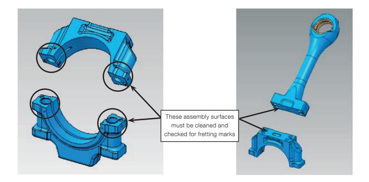
After cleaning the assembly surface at the connecting rod/marine head and the assembly surfaces of the upper and lower marine head parts should be checked for fretting marks.
