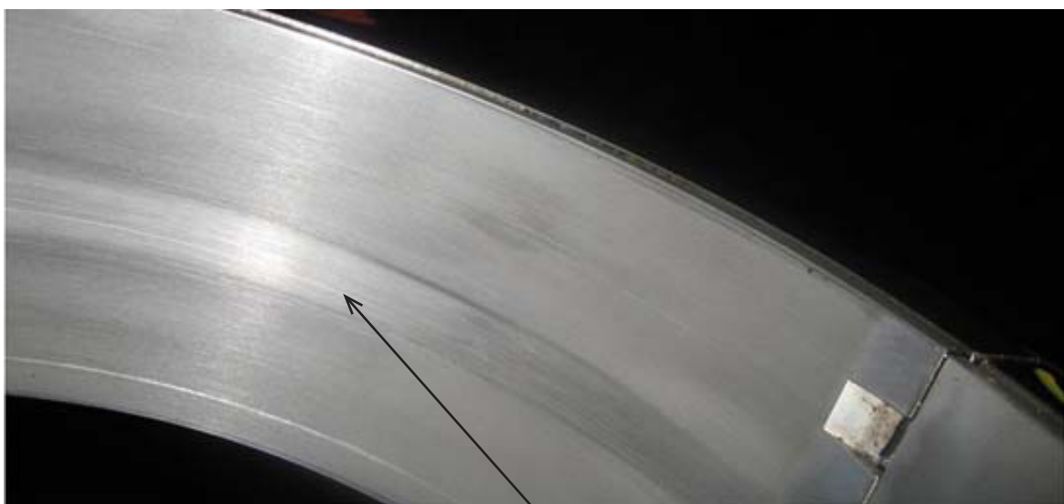
Bearing shell with damage from ridge wear.
