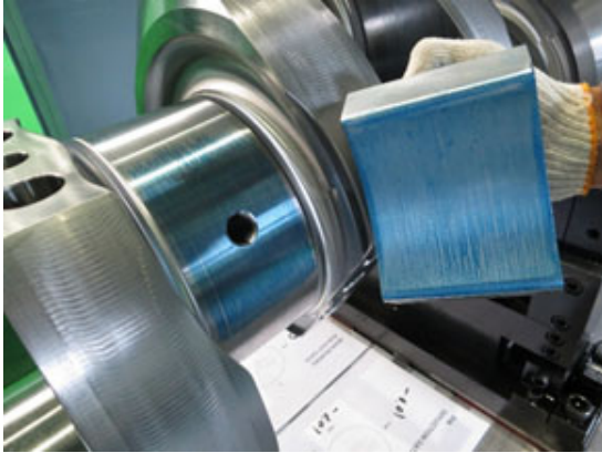
Test with test shell in workshop
