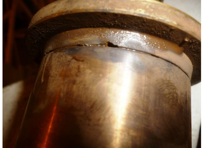
Corrosion / cavitation on sealing surface
