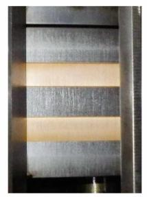
Bronze bands worn flush, but chamfers in fine condition.
